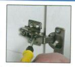
As shown, the screw the screwdriver points to, Itmoves the door from side to side, Clockwise rotation is to adjust the door panel to the middle
